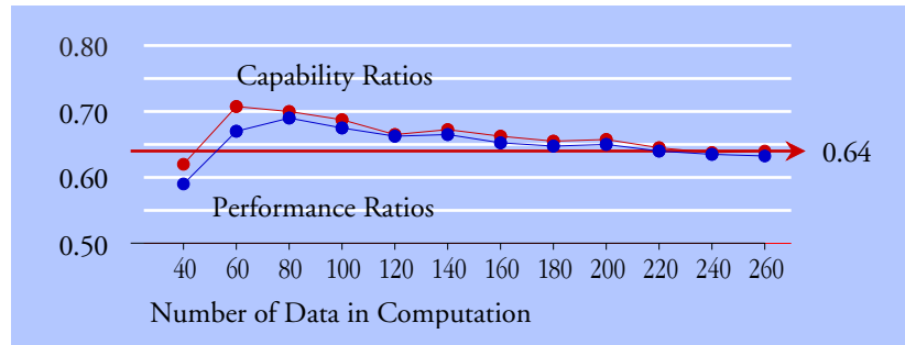
Figure 6: Performance and Capability Ratios for Example One Converge with Increasing Amounts of Data
