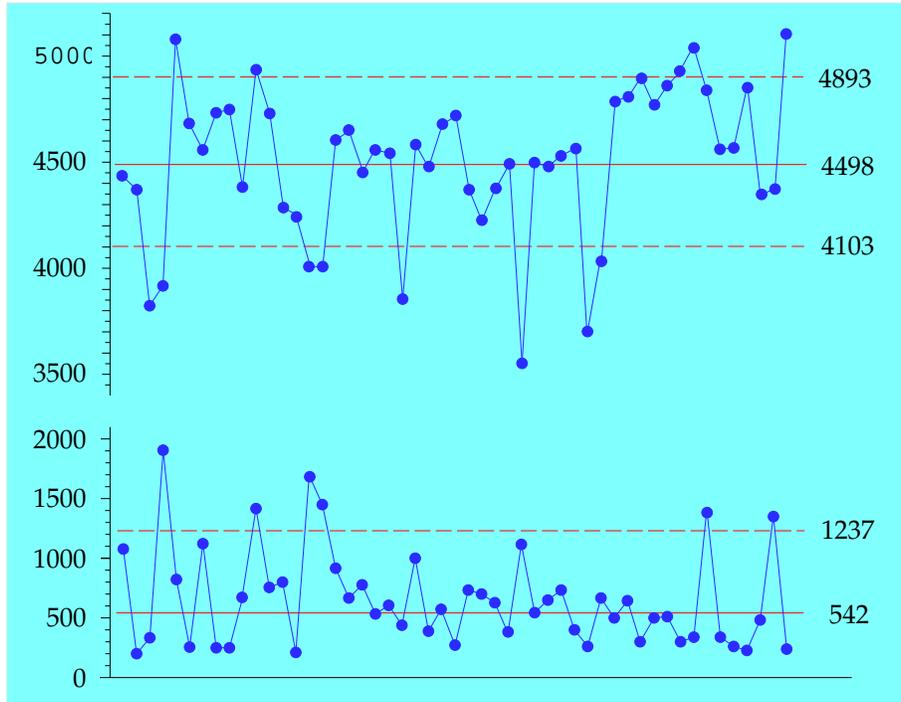
Figure 2: Resistivity Data with Limits Based on Revised Average Range
