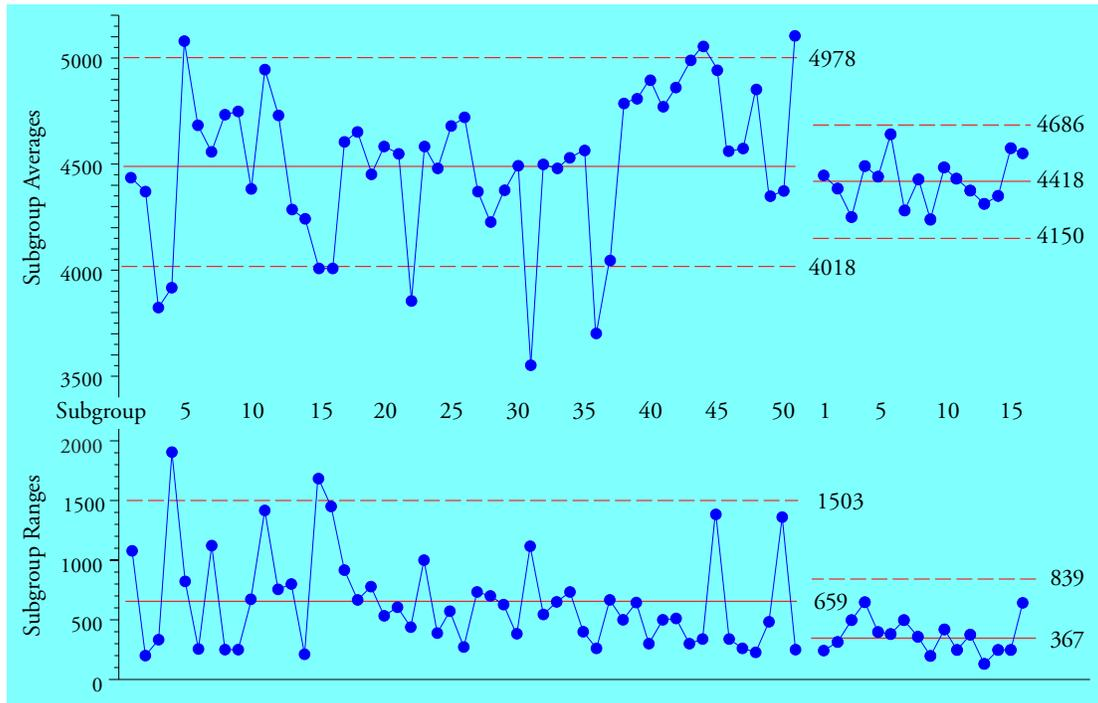
Figure 4: Resistivity Data Before and After Discovery of Assignable Cause
