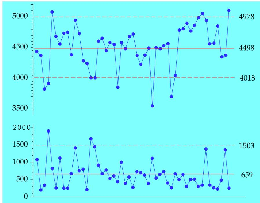
Figure 1: Resistivity Data with Original Limits
